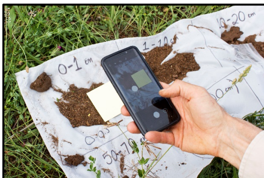
Figure 14: Determining soil color using a soil app on a smartphone
