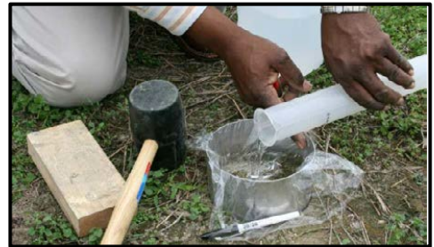
Figure 7: Preparing soil infiltration test
